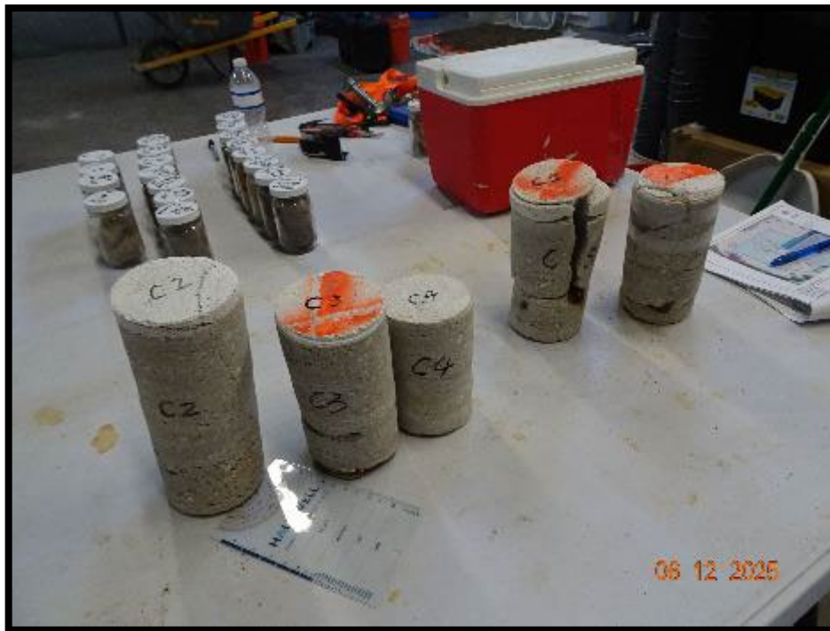
Photo 10 View of core samples taken by Pacscon in their lab. Note cracked cores along C1, C5 and C2. C5 had the severe crack with corroded reinforcement.
